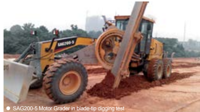
● SAG200-5 Motor Grader in blade-tip digging test
