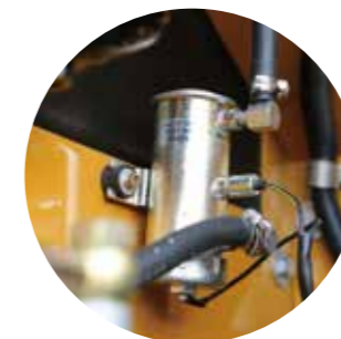
Electronic oil pump will pump oil automatically after the filter element is maintained.
